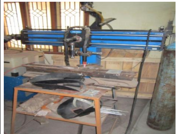
Figure 3: TIG Welding Set-Up
