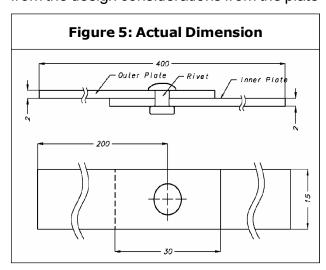
thickness as 2 mm and that are specified in the following diagram. Figure 5 shows the configuration, dimensions, constraints and loading conditions. The following assumptions and boundary conditions were considered throughout the idealization process:
