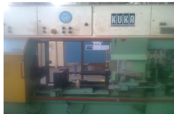
Figure 1: KUKA Friction Welding Machine (WRI, BHEL)
