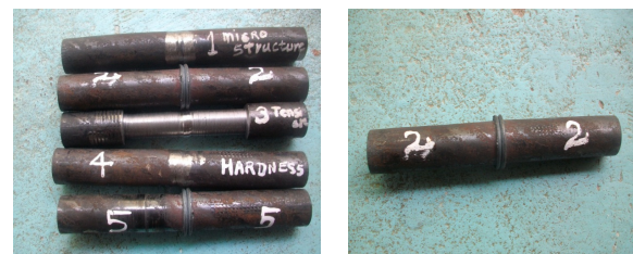
Figure 2: Friction Welded Joints of EN-24 Cylindrical Rods
