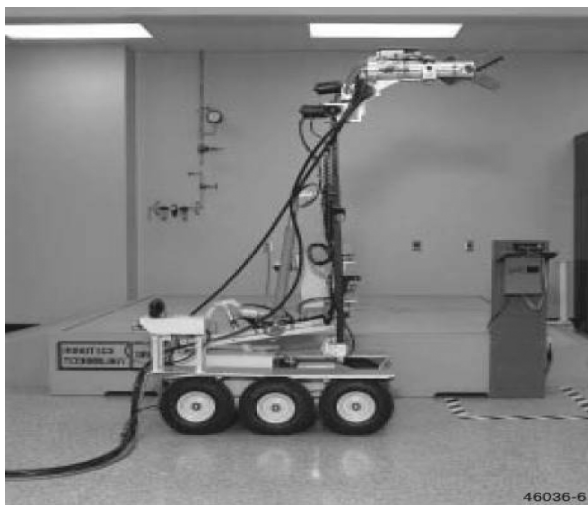
Figure 7: Mobile Teleoperator Used to Remove a Wall-Mounted Junction Box
