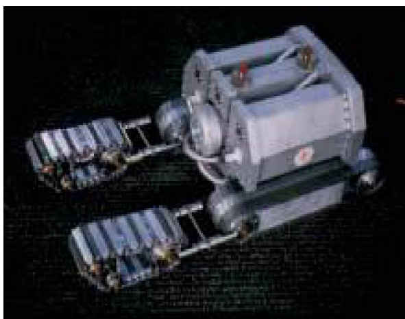
Figure 4: Neptune In-Tank Crawler Robot
