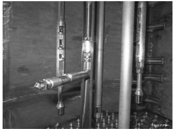
Figure 8: Reactor Tank Inspection Robot
