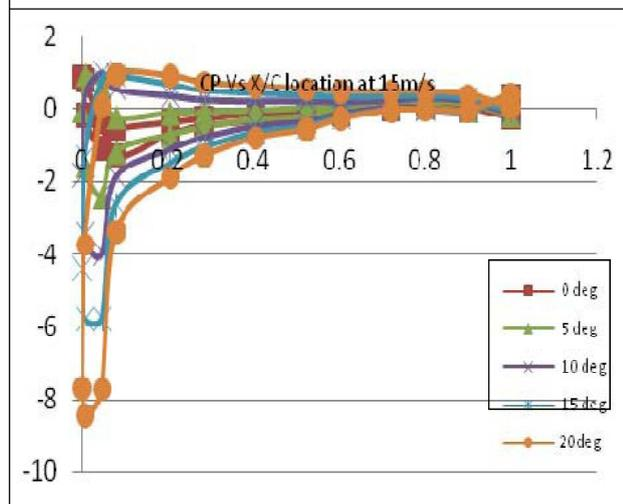
**Figure 6: Coefficient of Pressure on Upper Surface at Velocity 15 m/s at Various Angle of Attack 0 to 20 Degree**
