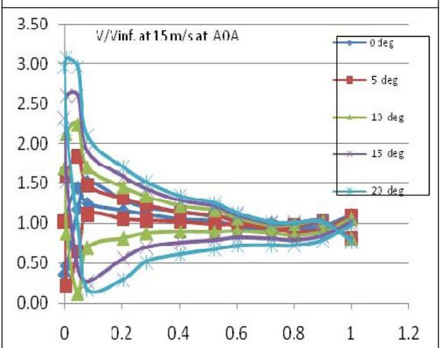
**Figure 9: Shows the Velocity Ratio at Upper Surface of an Airfoil**
