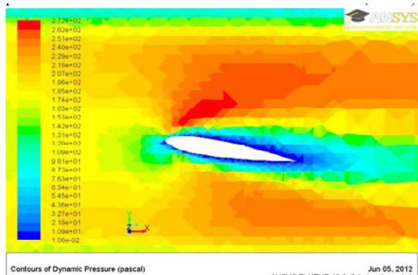
**Figure 14: Shows that Pressure Distribution Over the Airfoil at Velocity 12 M/S Angle of Attack 10 Degree Contours of Total Pressure (Pascal)**
