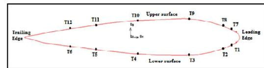
Tygon tubes are inserted in these tap holes for measurement of gauge pressure by connecting with multi-tube manometer.
