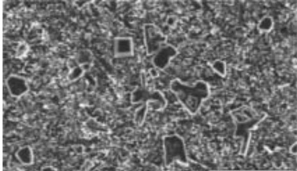
**Figure 5: SEM Image of the Eutectic Mixture of the Two Alloys at a Magnification of 5000X (a) Al-17%Si-0.5Mg-4%Ba (b) Al-17%Si-0.5Mg-5%Ba**
