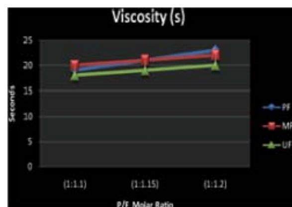
Figure 1: Variation of Viscosity with Increase in P/F Molar Ratio in Different Resins
