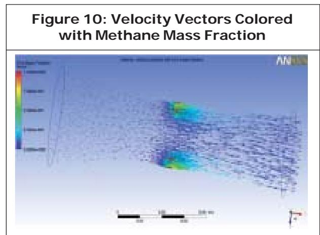
As inlet air flows toward the engine, a maximum negative pressure is produced at the throat of the venturi (Anil *et al.*, 2006). The gaseous fuel, adjusted and held in a pressure to a large extent equal or near atmospheric pressure (in this case, 34.47 kPa) by the help of a regulator is installed between the gas cylinders and the carburetor fuel inlet.
