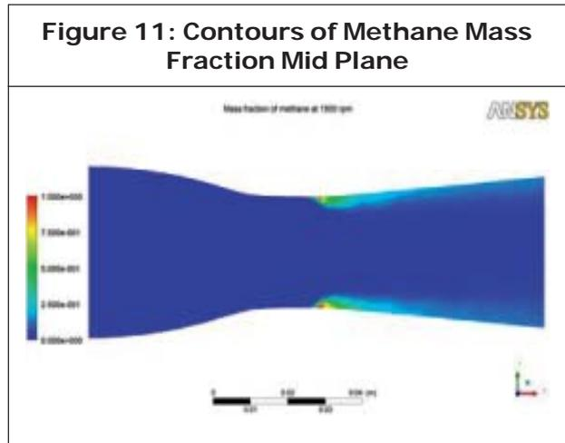
Above graphs shows that the mixture is rich in the regions close to the walls and on the contrary, mixture is quite lean near the axis of the carburetor.
