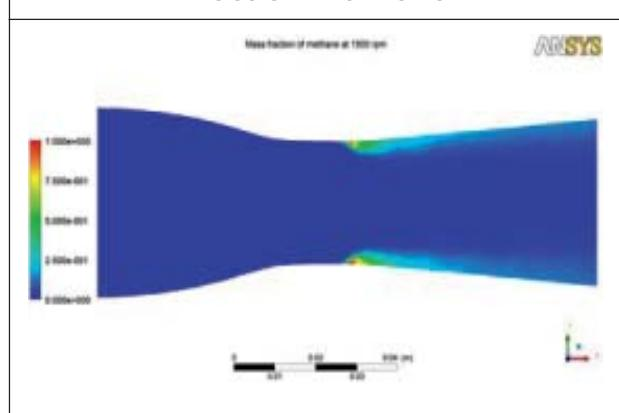
Above graphs shows that the mixture is rich in the regions close to the walls and on the contrary, mixture is quite lean near the axis of the carburetor.
