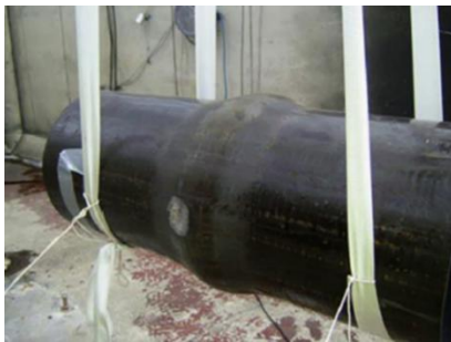
Fig. 5. Test cylinder suspended from sling after internal explosive loading (0.6 kg TNT) [23].
