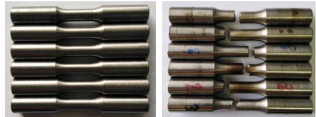
Fig. 14. S45C steel was used for fatigue testing before and after the experiment.
