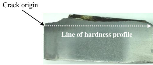
Fig. 12. The failed drive shaft hardness measurement line is measured from the case to the core of the shaft.
