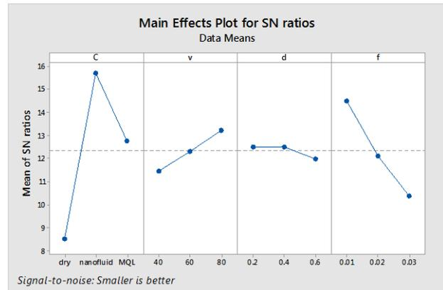
Fig. 2. The S/N ratio plot for surface roughness.
