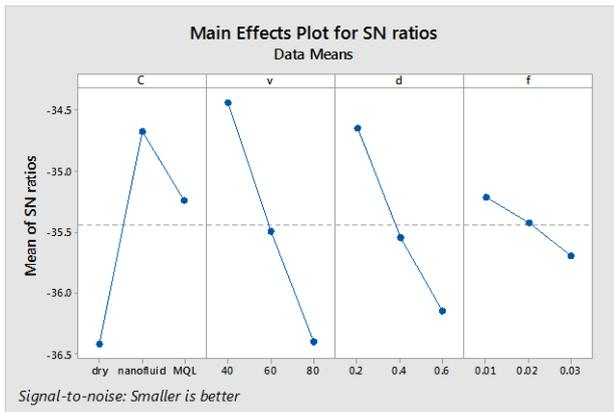
Fig. 6. The S/N ratio plot for the cutting temperature.
