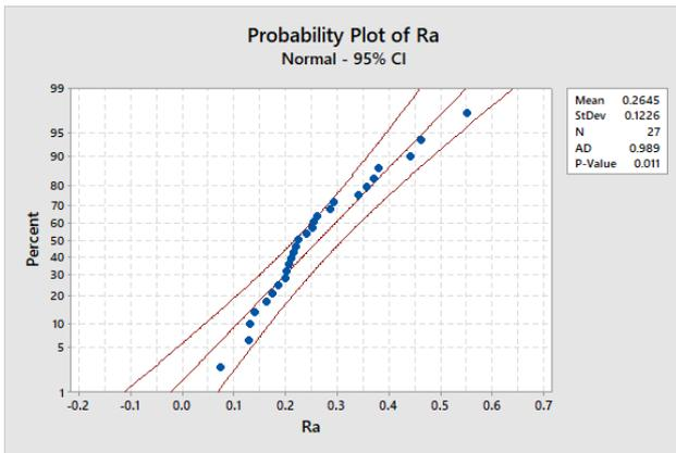
Fig. 3. The surface roughness probability plot.
