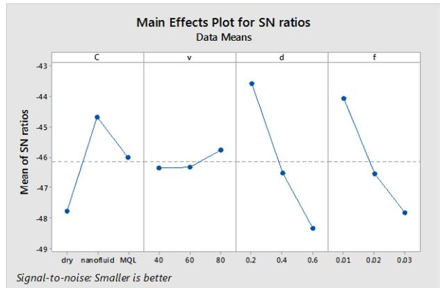
Fig. 4. The S/N ratio plot for cutting force.
