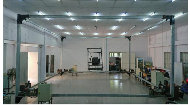
Figure 1. Cable Robot with 8 cables, 6 dof.
