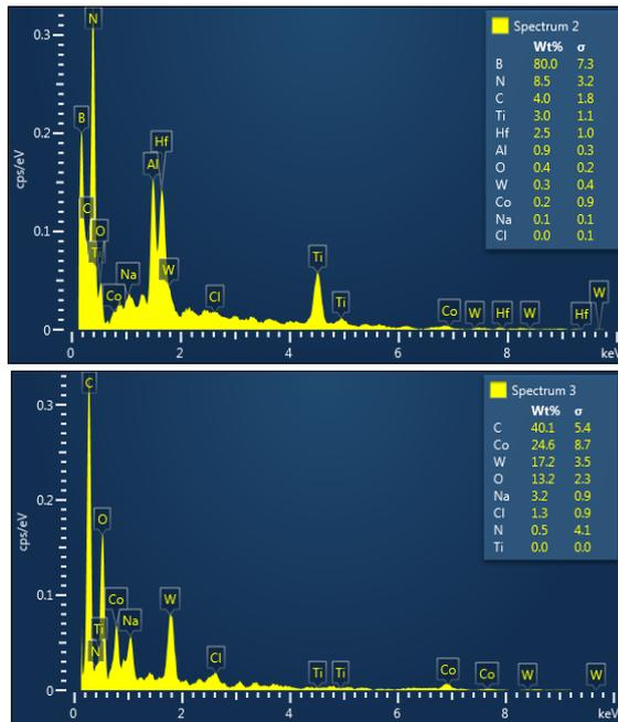
Figure 10. The EDS analysis results for the experiment 3
