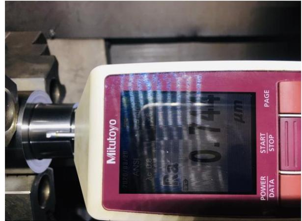
Figure 2. The surface roughness tester
