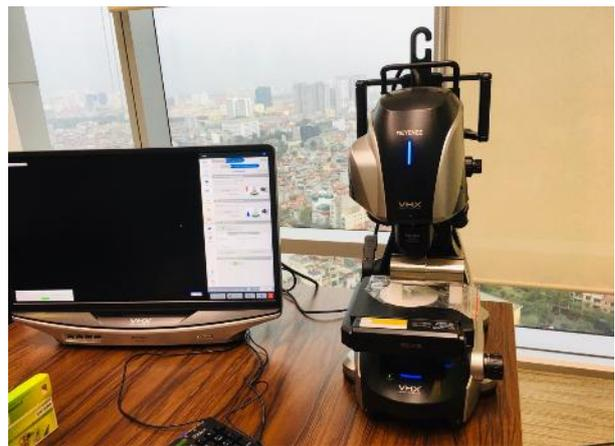
Figure 3. Digital microscope VHX-7000 by Keyence
