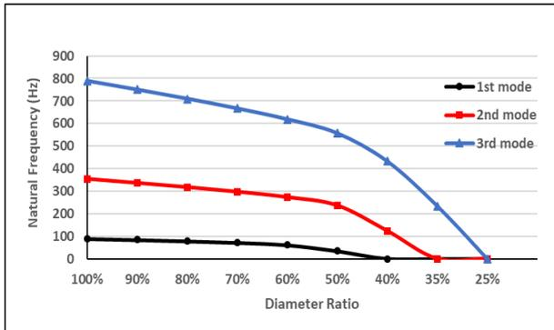
Figure 4. First three natural frequencies versus the outlet/inlet diameter ratios for fluid flow velocity 5 m/s.
