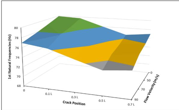
Figure 12. Effect of crack position and fluid velocity on the first fundamental circular frequencies of tapered simply supported pipe for crack depth 7mm.
