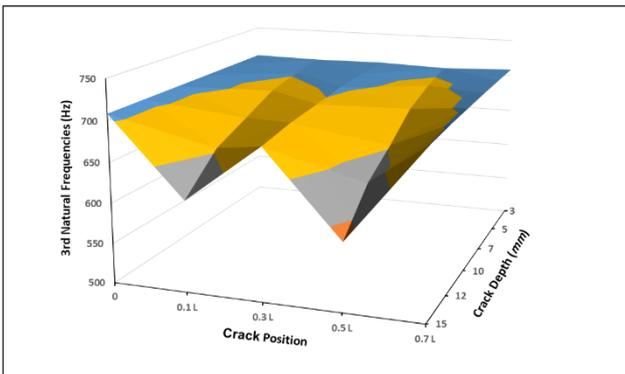
Figure 8. Effect of crack depth and crack position on the third circular frequency of tapered simply supported pipe for fluid flow velocity 10 m/s.
