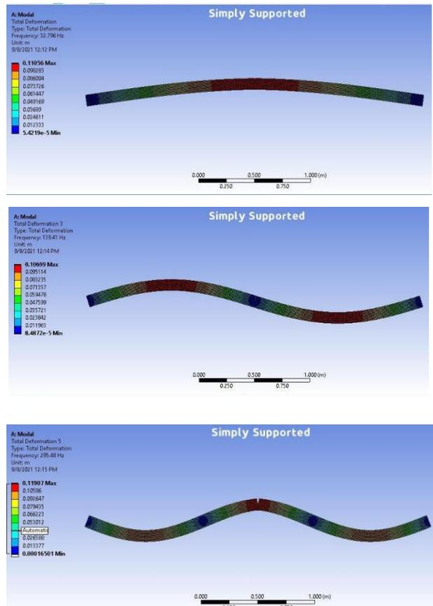
Figure 5. Mode shapes for first three fundamental frequencies for the tapered hinged pipe conveying fluid.
