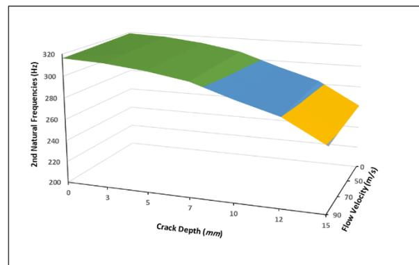
Figure 10. Effect of crack depth and fluid velocity on the second circular frequencies of tapered simply supported pipe for crack relative position 0.3 L.
