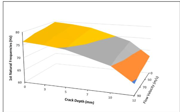
Figure 9. Effect of crack depth and fluid velocity on the first circular frequencies of tapered simply supported pipe for crack relative position 0.3 L.
