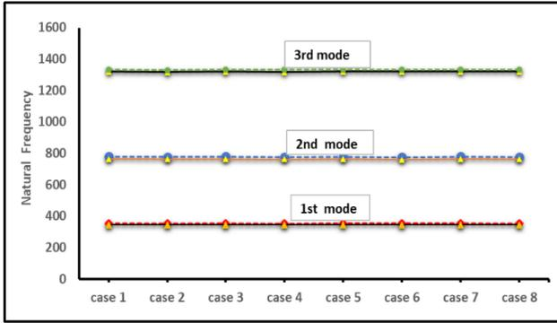
Figure 3. Comparison of first three natural frequencies for the uniform cross-section with double cracks for different cases.
