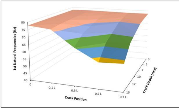
Figure 6. Effect of crack depth and crack position on the first circular frequency of tapered simply supported pipe for fluid flow velocity 10 m/s.
