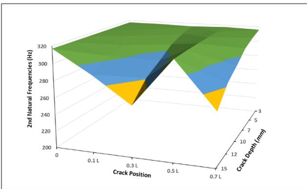
Figure 7. Effect of crack depth and crack position on the second circular frequency of tapered simply supported pipe for fluid flow velocity 10 m/s.
