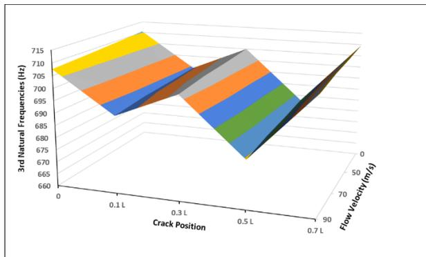
Figure 14. Effect of crack position and fluid velocity on the third fundamental circular frequencies of tapered simply supported pipe for crack depth 7mm.
