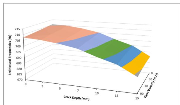
Figure 11. Effect of crack depth and fluid velocity on the third circular frequencies of tapered simply supported pipe for crack relative position 0.3 L.
