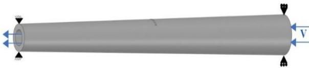
Figure 1. Schematic illustrating fluid conveyance via a hinged pipe with a changing cross section.
