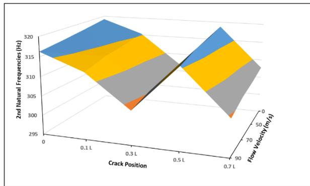
Figure 13. Effect of crack position and fluid velocity on the second fundamental circular frequencies of tapered simply supported pipe for crack depth 7mm.
