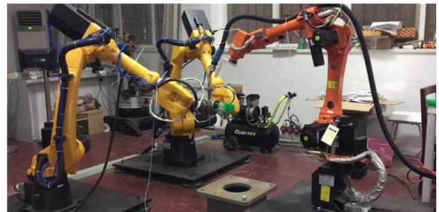
Figure 1. Example of multi-robot cooperation in a welding task [1].
